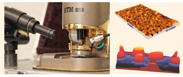
Scanning Tunneling Microscope (STM) & Results
